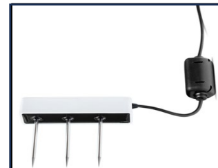
Soil moisture sensor clusters+ manual measurements
